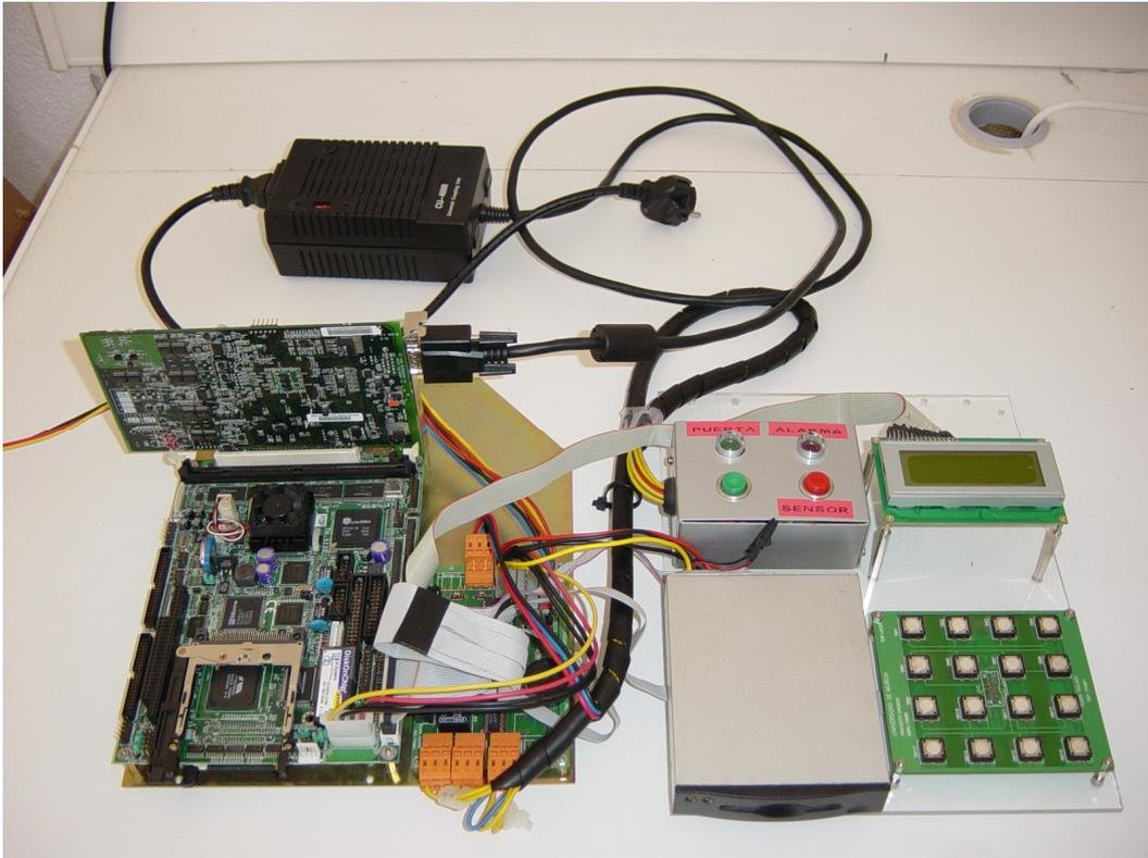
**Figure 2-1: PLC-UMU Home Automation Device**
