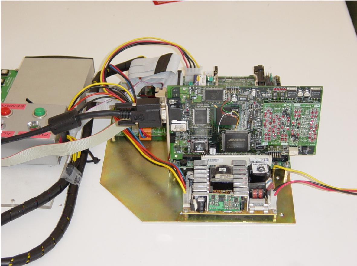
Figure 2-3: PCI PLC Card and Device's Main Board (II)
