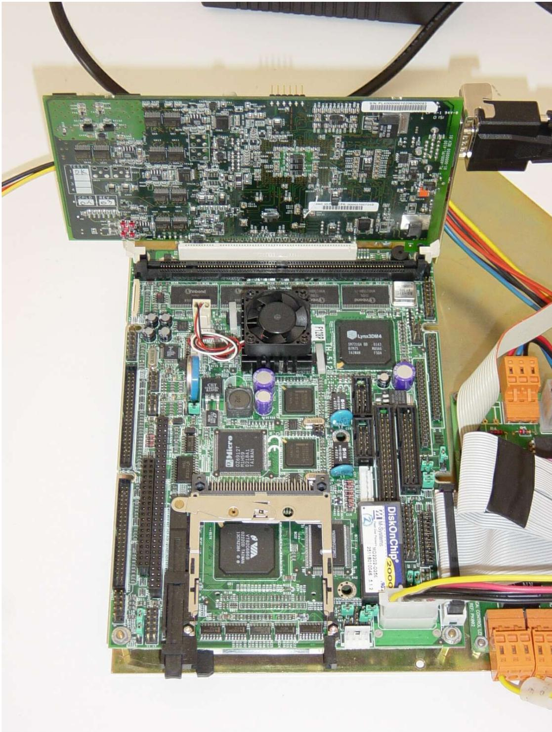
**Figure 2-2: PCI PLC Card and Device's Main Board (I)**
