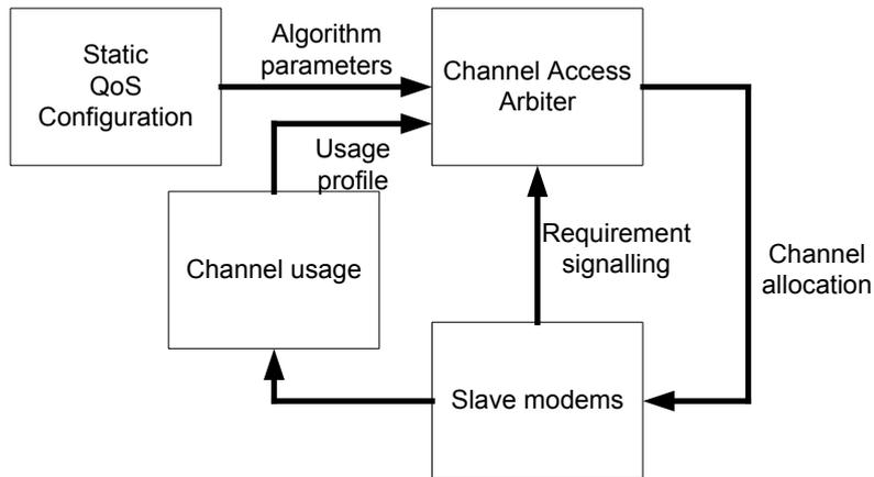
**Figure 3-3: Static QoS Configuration**
