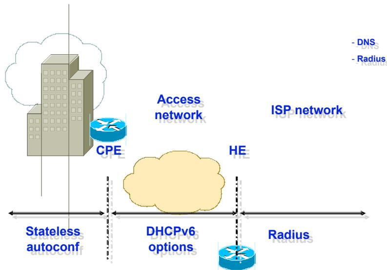
Figure 2-1: Autoconfiguration Overview
