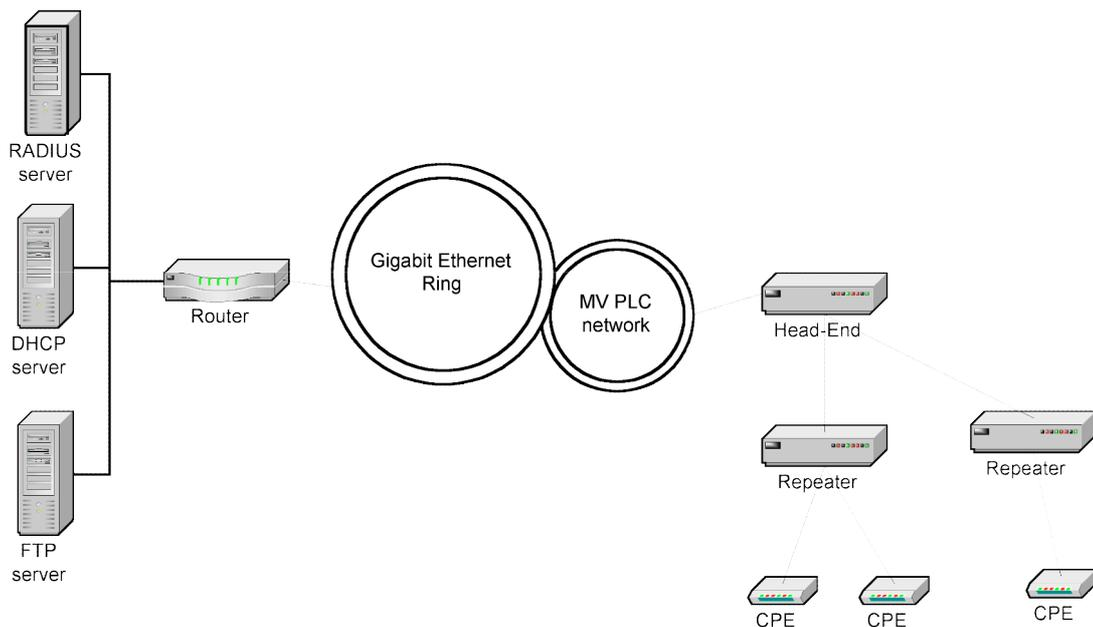
**Figure 3-1: Elements Involved in the Autoconfiguration Process**
